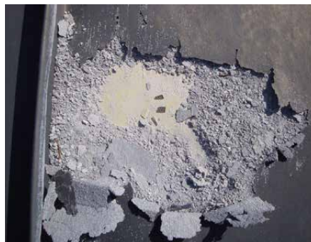
The effect of back side corrosion on zinc.
